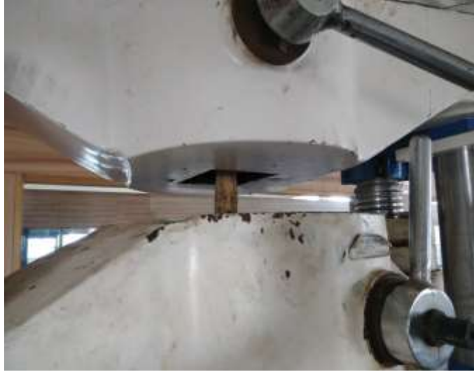
Figure 4.2 Grip components for tensile test
