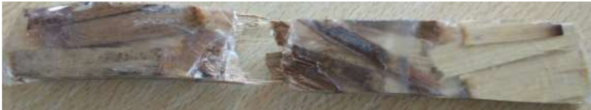
Figure 4.6 Specimen after flexural test
