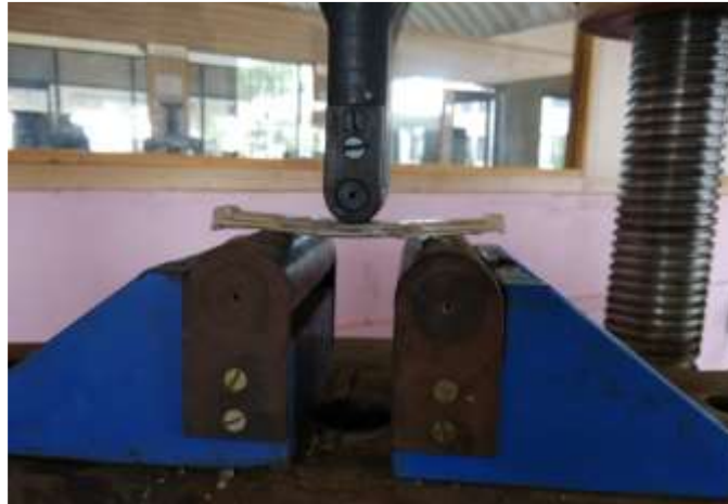
Figure 4.5 Grip components for flexural test
